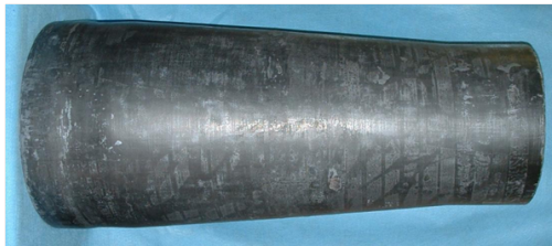
CMC combustor liner
